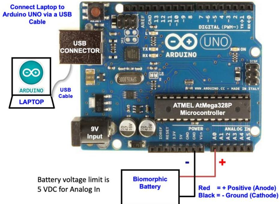
Fig 6: The Arduino to measure the battery voltage.
