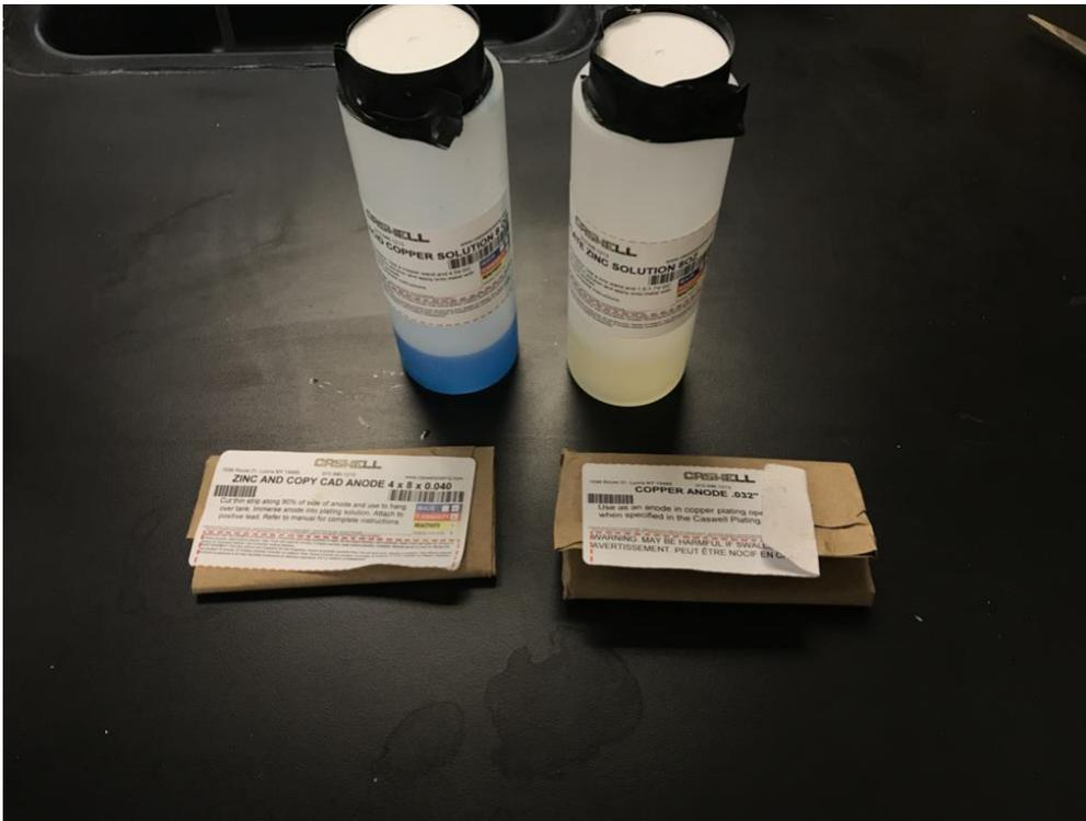
Fig 3: Zinc and Copper solutions with their respective metals.
