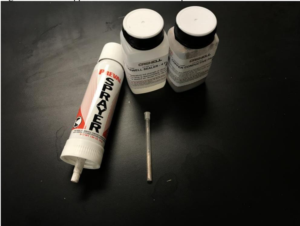
Fig 4: The copper conductive paint for the stems to be covered in.
