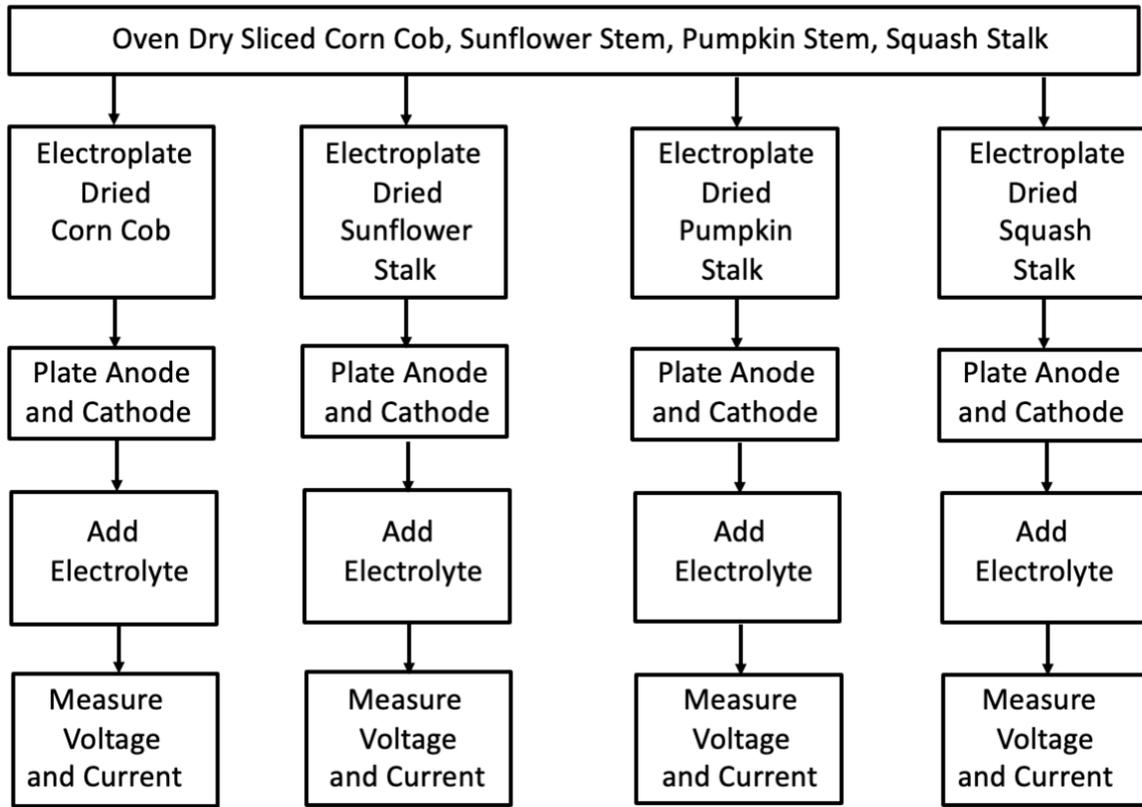
Fig 5: Flow chart for electroplating the Biomorphic Battery
