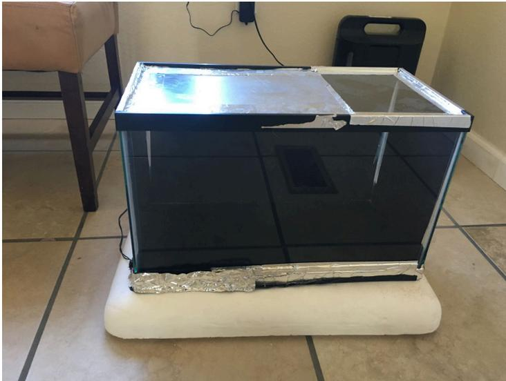
Cloud Chamber experiment, one by one, places chosen shielding materials within the cloud chamber over the radiation source in a manner that will make it easy to distinguish if the shielding materials are blocking radiation particles from the source. With each material, count and identify the radiation particle trails, the alpha, beta, or gamma interactions. Fig. 6. Note: Cloud Chamber is used strictly for visual purposes.
